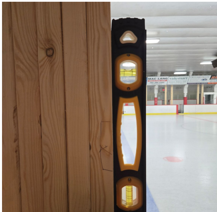
Photograph 8: Marked post and level check at representative monitoring location
